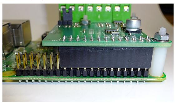
This means: The pin header socket actually does not hit the socket base of the pin header, but the contacts will have sufficient overlap.
