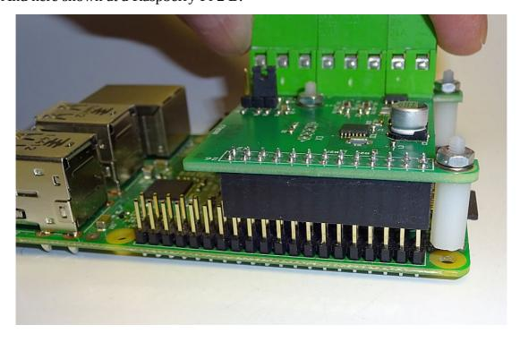
Now the PiLogger PCB has to be pressed down gently until the stand off's touch the Raspberry Pi PCB.
