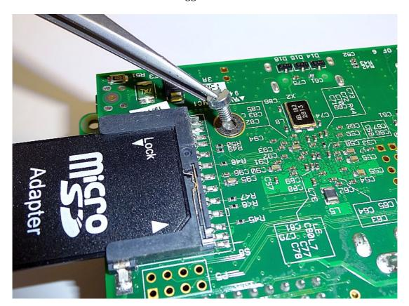
Subsequently we turn in one screw to each stand off by hand and not too tight, so they fit accurately without any bending in case there are 2 of them. Subsequently we tighten them by using a screw driver just moderate:
